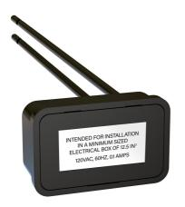
Designed to improve dimmer performance, use this bypass module in applications where flickering or ghosting (when a low level of light is emitted even in the "off" position) occur. As an LED dimming load adapter, the module is usable with most 120V dimmers and makes for easier troubleshooting with ultra-low wattage LED lights. Can be wired into most electrical wall boxes (if neutral wire is present) or right at the light fixture.
