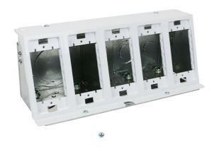
Bank of five (5) compartments that accept power, communications and audio/video devices. Accepts EFB10 Series device plates (2 1/32'' x 4 5/8'') (58mm x 117mm). Includes one mounting bracket, one back plate, one divider, two (2) end caps and two (2) knockout plates. Device plates sold separately. NOTE: Module will fit on either side of the floor box.
