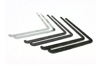
Used for floor coverings greater than 3/6'' (4.7mm). The EFB45-TS allows the finished cover assembly to be flush with the finished floor. Includes one (1) 1/16'' (1.6mm), one (1) 1/8'' (3.2mm) and one (1) 1/4'' (6.4mm) tile shims for 7/16'' (11.1mm) of upward adjustment.
