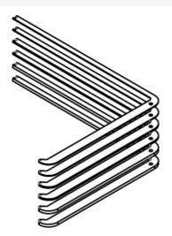
Used for floor coverings greater than 3/16" (4.7mm). This tile shim allows the finished cover assembly to be flush with the finished floor. Includes one (1) 1/16" (1.6mm), one (1) 1/8" (3.2mm) and one 1/4" (6.4mm) tile shim for 9/16" (14.3mm) of upward adjustment.
