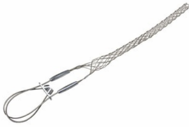
FC050LB: Standard Duty, Closed Mesh, Locking Bale (Universal Eye), Cable Diameter 0.50 - 0.61 inches, Bale Length 18-in, Mesh Length 11-in, Break Strength 770 lbs.
