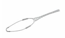
FC100U: Standard Duty, Closed Mesh, Single-Eye Grip, Cable Diameter 1.00 - 1.24 inches, Bale Length 9-in, Mesh Length 15-in, Break Strength 1680 lbs.
