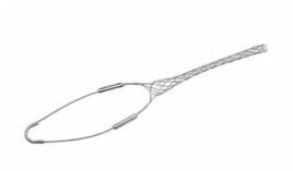
FC125U: Standard Duty, Closed Mesh, Single-Eye Grip, Cable Diameter 1.25 - 1.49 inches, Bale Length 10-in, Mesh Length 16-in, Break Strength 1680 lbs.
