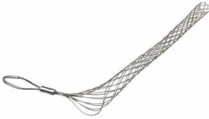
FC2000F: Standard Duty, Closed Mesh, Offset Eye Grips, Cable Diameter 2.00 - 2.49 inches, Bale Length 6-in, Mesh Length 22-in, Break Strength 3760 lbs.
