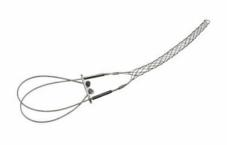
FC300LB: Standard Duty, Closed Mesh, Locking Bale (Universal Eye), Cable Diameter 3.00 - 3.49 inches, Bale Length 18-in, Mesh Length 26-in, Break Strength 5280 lbs.
