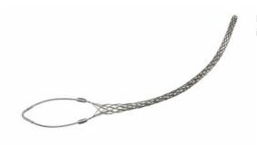
FCHL125U: Standard Duty, Closed Mesh, Single-Eye Grip, Cable Diameter 1.25 - 1.49 inches, Bale Length 10-in, Mesh Length 31-in, Break Strength 4720 lbs.
