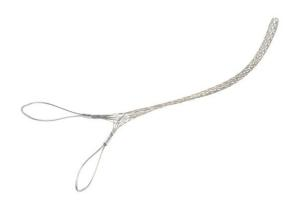
FCHL250UU: Heavy-Duty, Closed Mesh, Double-Eye, Cable Diameter 2.50 - 2.99 inches, Bale Length 10-in, Mesh Length 39-in, Break Strength 10080 lbs.
