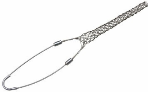
FCSD52: Service Drop, Closed Mesh, Single Eye, Cable Diameter 0.53 - 0.73 inches, Bale Length 8-in, Mesh Length 8-in, Break Strength 790 lbs.
