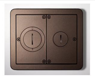
Flanged cover for use in tile or carpet installation. Die-cast aluminum assembly. Provided with one 1" trade size screw plug for power or communication type cabling and one combination 1 1/4" and 2" trade size screw plug for communication type cabling. Allows for feeding both power and communication cabling. NOTE: Add suffix "TR" to the end of the part number to indicate tamperresistant cover assembly. Tamper-resistant versions are secured with a single tamper-resistant screw.
