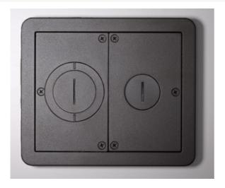
Flanged cover for use in tile or carpet installation. Die-cast aluminum assembly. Provided with one 1in trade size screw plug for power or communication type cabling and one combination 1 1/4in and 2in trade size screw plug for communication type cabling. Allows for feeding both power and communication cabling. NOTE: Add suffix "TR" to the end of the part number to indicate tamperresistant cover assembly. Tamper-resistant versions are secured with a single tamper-resistant screw.
