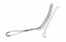
FR0500F: Standard Duty, Split Rod, Offset Eye, Cable Diameter 0.50 - 0.61 inches, Bale Length 4-in, Mesh Length 11-in
