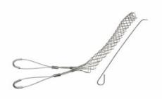
FR062UU: Standard Duty, Split Rod, Double-Eye, Cable Diameter 0.62 - 0.74 inches, Bale Length 4-in, Mesh Length 11-in, Break Strength 960 lbs.
