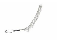
FR1250F: Standard Duty, Split Rod, Offset Eye, Cable Diameter 1.25 - 1.49 inches, Bale Length 5-in, Mesh Length 16-in
