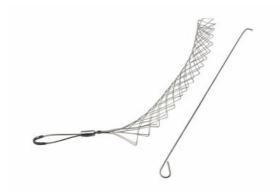
FR1500F: Standard Duty, Split Rod, Offset Eye, Cable Diameter 1.50 - 1.74 inches, Bale Length 5-in, Mesh Length 18-in
