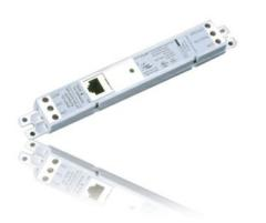
The FS-PP Fixture Power Pack provides 24 VDC operating voltage to the FS Low Voltage Sensor series via the RJ45 connector built onto each sensor. The incorporated Form-C Relay, Normally Open (N/O)/Normally Closed (N/C), can control line or low voltage loads.
