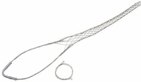
FS062U: Standard Duty, Split Lace, Single Eye, Cable Diameter 0.62 - 0.74 inches, Bale Length 8-in, Mesh Length 11-in, Break Strength 960 lbs.
