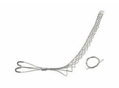
FS100UU: Standard Duty, Split Lace, Double-Eye, Cable Diameter 1.00 - 1.24 inches, Bale Length 5-in, Mesh Length 15-in, Break Strength 1920 lbs.
