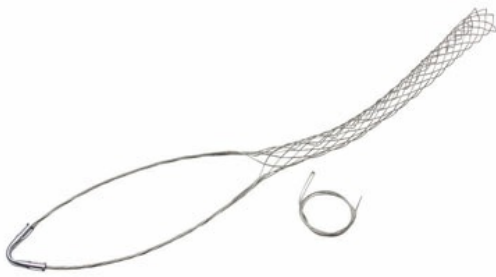
FS150U: Standard Duty, Split Lace, Single Eye, Cable Diameter 1.50 - 1.74 inches, Bale Length 12-in, Mesh Length 18-in, Break Strength 1680 lbs.
