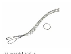
FS175UU: Standard Duty, Split Lace, Double-Eye, Cable Diameter 1.75 - 1.99 inches, Bale Length 6-in, Mesh Length 20-in, Break Strength 3150 lbs.
