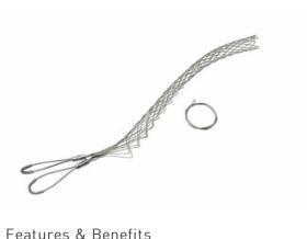
FS200UU: Standard Duty, Split Lace, Double-Eye, Cable Diameter 2.00 - 2.49 inches, Bale Length 6-in, Mesh Length 22-in, Break Strength 3360 lbs.
