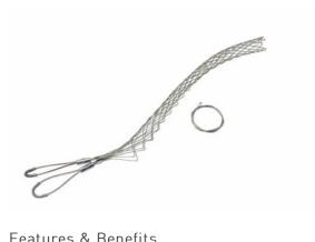
FS250UU: Standard Duty, Split Lace, Double-Eye, Cable Diameter 2.50 - 2.99 inches, Bale Length 6-in, Mesh Length 24-in, Break Strength 3360 lbs.
