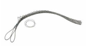
FSHL100UU: Heavy-Duty, Split Lace, Double-Eye, Cable Diameter 1.00 - 1.24 inches, Bale Length 10-in, Mesh Length 29-in, Break Strength 4720 lbs.
