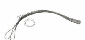
FSHL300UU: Heavy-Duty, Split Lace, Double-Eye, Cable Diameter 3.00 - 3.49 inches, Bale Length 10-in, Mesh Length 41-in, Break Strength 10080 lbs.
