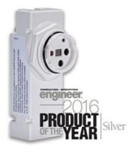
The FSP-201 mounts in an outdoor lighting fixture and provides multi-level control based on motion and/or daylight contribution. It controls 0-10 VDC dim-to-off LED drivers or ballasts, or works with a power pack to control other loads. When used with an FSP-Lx Lens, the sensor is rated for wet and cold locations. All control parameters are adjustable via a wireless configuration tool capable of storing and transmitting sensor profiles.
