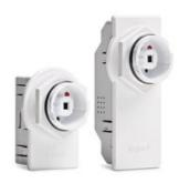
FSP-2x2 sensors provide multi-level control based on motion and/or daylight contribution. They control 0-10VDC LED drivers or dimming ballasts, as well as non-dimming ballasts and, with an FSP-Lx Lens, are rated for wet and cold locations. Line and low voltage models are available, and choice of control modes simplifies sensor configuration.
