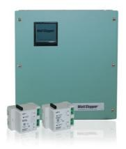
The LC8 panel provides zone-based control of up to eight channels, or zones, of interior and exterior lighting. Zones respond to control signals from the system clock, or an accessory photocell, to automatically turn lighting on and off. The LC8 panel uses interchangeable relay modules, available separately, that can be selected to suit project needs. Relay options include the LCSP-2 dual single-pole module and LCDP1 double-pole module.
