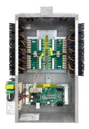
The LMCP series panels are available for Dimming (LMCPx-10V) or Switched(LMCPx) control of lighting and plug loads. The panels can be networked together to enable automation through out an entire facility. The HDR panel relays respond to inputs from Digital Lighting Management (DLM) switches, occupancy sensors, daylight sensors, input modules and 0-10V outputs on dimming panel models.
