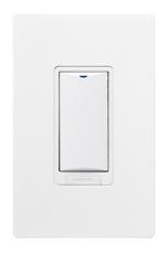
The LMDM-601 Dimming Wall Switch is a wireless low voltage device for dimming control of one or more lighting loads. It is part of the wireless Digital Lighting Management (DLM) system and can dim load(s) connected to wireless DLM dimming room controllers (LMRC-611) for a totally wireless room. Alternatively it can be used in a hybrid wired & wireless room to control loads connected to a traditional wired room controller (e.g. LMRC-111) when used in conjunction with a wireless bridge (LMBC-650).
