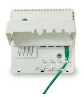
LMPL-201 Plug Load Controllers include a 20 amp relay for on/ off control of connected outlets, and a high-efficiency switching power supply. They are part of a Wattstopper Digital Lighting Management (DLM) system, and enable energy-efficient control of plug loads.
