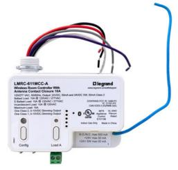
The LMRC-611MCC is a wireless DLM room controller, part of the foundation of the wireless Digital Lighting Management (DLM) system which includes occupancy sensors, daylighting controls, and switches for energy-efficient control. The LMRC-611MCC includes one relay to switch a total of 10 amps, a high-efficiency switching power supply, and both Class 1 and Class 2 0–10 volt outputs for control of dimmable loads including compatible LED drivers and electronic ballasts.
