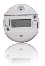
The LS-102 Daylighting Controller is a single zone, on/off switching device designed to be installed in a closed loop application. A self-contained 24 VDC device with an extended range of 1-1400 footcandles, the LS-102 requires a low voltage power pack to operate. The controller consists of an advanced digital multi-band photosensor, an on-board microcontroller, and an LCD display. This photosensor is positioned behind a 100° cone that cuts off unwanted light, preventing false triggers.
