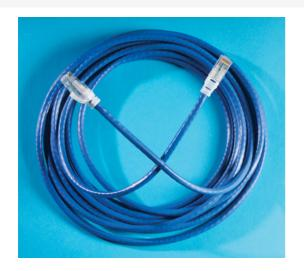
Clarity 6 Modular Patch Cord, blue, 15', Category 6, four-pair UTP stranded 24 AWG PVC/CM, center tuned with Clarity 6 connecting hardware for optimum Category 6 installed performance using Ortronics Paralign 2 pair-positioning technology.
