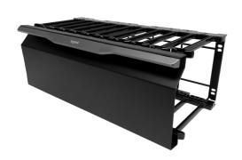
Horizontal cable managers are available in 2RU and 4RU sizes. Fingers begin 3/4 in from the face of rack to provide bend limitation for cables, protecting cables, equipment and network performance. Included hinged cover mounts with six heavy duty clips allow them to be
