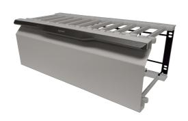
Horizontal cable managers are available in 2RU and 4RU sizes. Fingers begin 3/4 in from the face of rack to provide bend limitation for cables, protecting cables, equipment and network performance. Included hinged cover mounts with six heavy duty clips allow them to be
