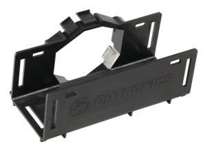
Universal cable troughs snap into the hex pattern on the Mighty Mo 20 channel racks and are used to create a front to rear or vertical trough on the inside or outside of the channel. They can be mounted in a row to create a continuous trough or rotated at 30° increments to support cables through directional changes. Up to 3 HiLOC™ harnesses can be toollessly mounted into each trough. The 2"x 2" size is equipped with slots to allow it to be joined to Mighty Mo Fiber Raceway.
