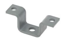
When ceiling support is required, ceiling hanger brackets are used with 5/8 in-11 in threaded rods and open or closed clips to suspend runway overhead.
