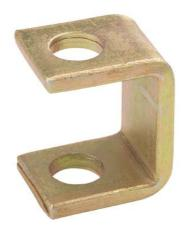
Use closed clips with 1-1/2 in stringers to secure runway to threaded rods when suspending runway from the ceiling. Also use when stacking runway. Use with 5/8 in-11 in threaded rod. Made of 1/4 in x 1-1/2 in steel bar. UL classified.
