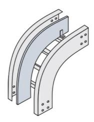
For extremely corrosive applications we offer a full line of straight sections, fittings, covers and mounting accessories in polyester and vinylester fiberglass. Rail heights are available in 4"" and 6"" and widths are available up to 36"".
