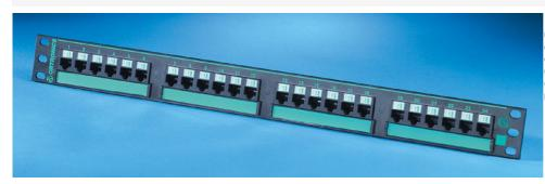
Clarity 5E 24-Port High Density Patch Panel is component compliant to EIA/TIA Category 5e performance requirements. It occupies one rack unit and measures 19" x 1.75". Jacks are grouped in six-port modules. Part of the Clarity 5E link and channel solution that provides significant installed performance headroom.
