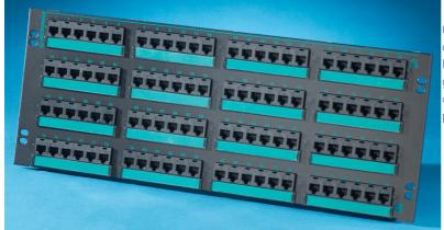
Clarity 5E 96-Port High Density Patch Panel is component compliant to EIA/TIA Category 5e performance requirements. It occupies four rack units, and measures 19" x 7". Jacks are grouped in six-port modules. Part of the Clarity 5E link and channel solution that provides significant installed performance headroom.
