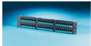
Clarity 5E 48-Port High Density Patch Panel is component compliant to EIA/TIA Category 5e performance requirements. It occupies two rack units, and measures 19" x 3.5". Jacks are grouped in eight-port modules. Part of the Clarity 5E link and channel solution that provides significant installed performance headroom.
