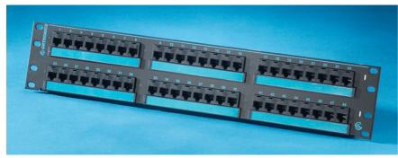
Clarity 6 48-Port High Density Category 6 patch panel is component compliant to EIA/TIA Category 6 performance requirements. It occupies two rack units and measures 19" x 3.5". Jacks are grouped in eight-port modules. Part of the Clarity 6 link and channel solution that provides significant installed performance headroom.
