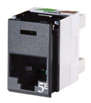
Clarity 5E panel jacks rear load into panels and exceed Category 5e component specifications. Rear load positive latch design, secures mounting of the jack into the panel. Universal T568A/B wiring label and tapered wiring towers simplify termination.
