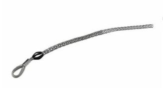
Medium Duty, Short Length, Flexible Eye, T-Type. Cable Diameter - 0.750-0.990-inch, Mesh Length - 24-inch, Eye Diameter - 1/4-inch, Break Strength - 6,800 lbs.
