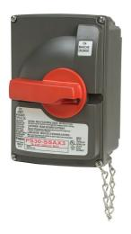
Non-Fusible Safety Switch with 3 Auxiliary Contacts, 30Amps, 600 VAC. The first non-metallic NEMA 4X Non-Fusible Safety Switch line UL Listed as Suitable as Motor Disconnect per NEC Article 430.109(A)(6). Pass and Seymour Non-Fusible Safety Switches feature extra-tough components, including an impact-resistant Valox NEMA 4X enclosure. And an innovative design that delivers safe, sure operation under the worst conditions.
