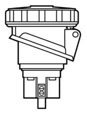
Double-Pole, Tamper-Resistant wire, Pin and Sleeve Receptacle. 100A, 250V.
